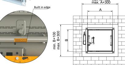
Drop rod and hanger location, please ensure that actuator operation is not compromised and ensure sufficient space to allow access hatch removal.
