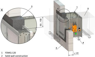
3 British gypsum thistle bond 60 (or equivalent can by used) minimum density 670 kg/m<sup>3</sup>
