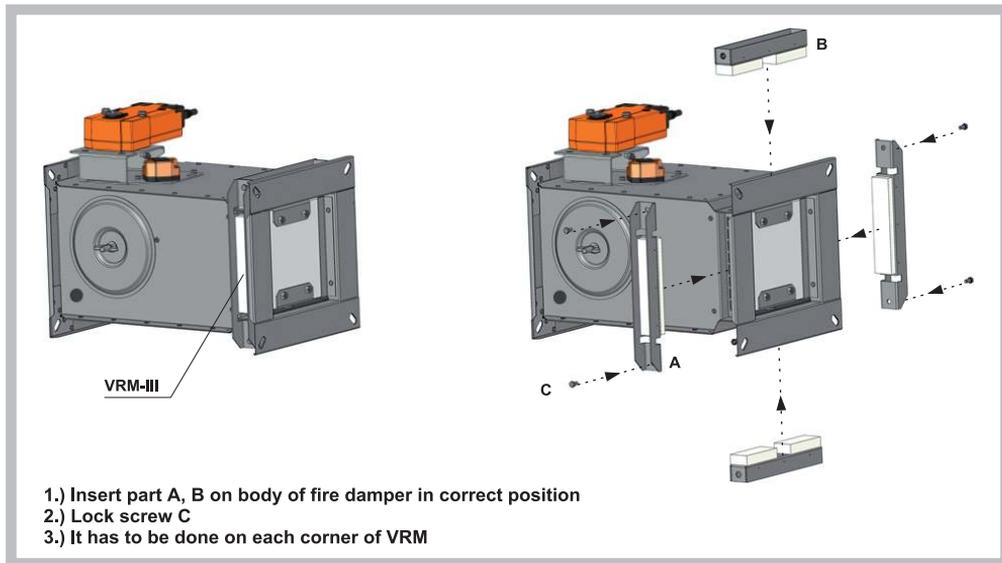
Notice: For installation outside of fire separating construction has to be used reinforcement VRM- III fixing.
