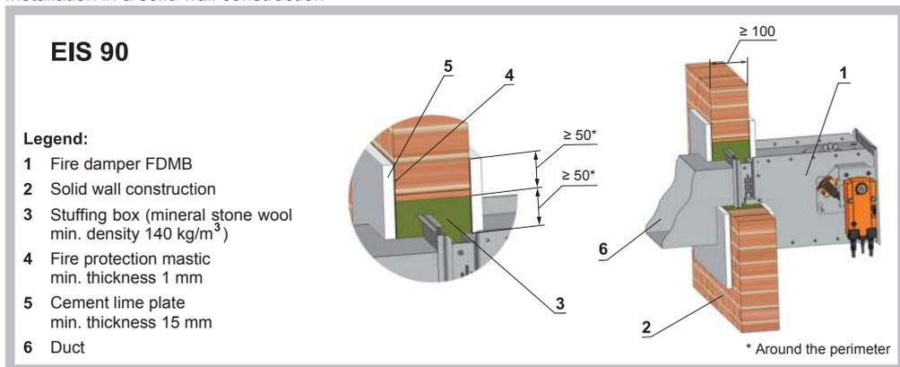
Installation in a solid wall construction (Weichschott system)
