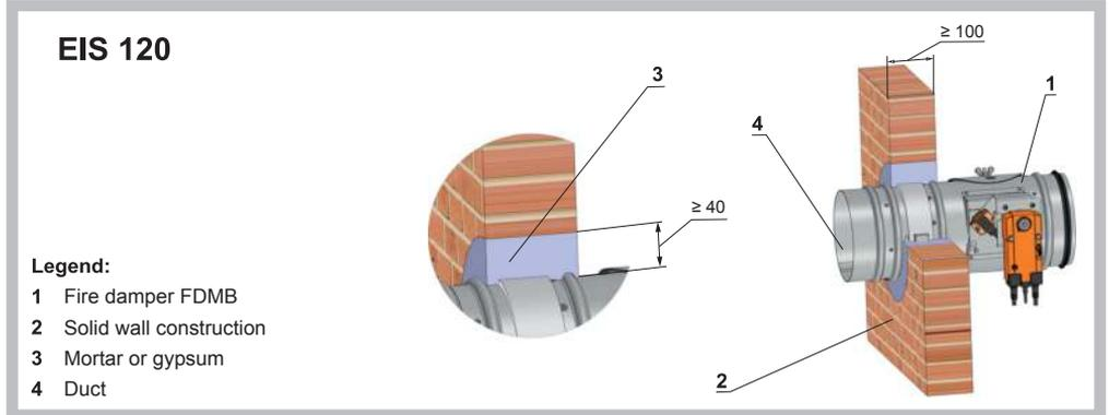
Installation in a solid wall construction
