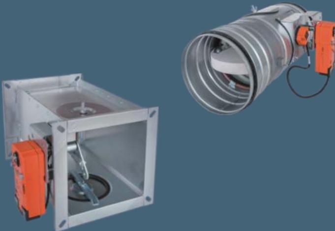
FIRE damper type FDMB, is in all variants classified: as **EI 120 ve, ho (i→o) S** or **EI 90 ve, ho (i→o) S** acc. EN 13501-3 and tested acc. EN 1366-2 and acc. EN 15650.
