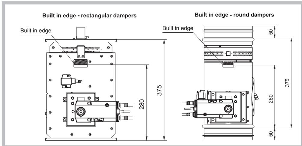
8. All fire dampers has to be closed during installation process. The damper body should not be deformed in the course of bricking in. Once the damper is built in, its blade should not grind on the damper body during opening or closing.
