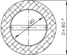
**Installation opening - round damper with actuating mechanism or manual and thermal**
