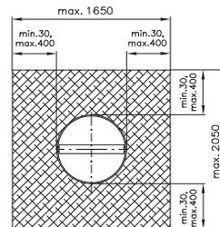
\* For damper with flange is the dimension  $D + 160$  mm
