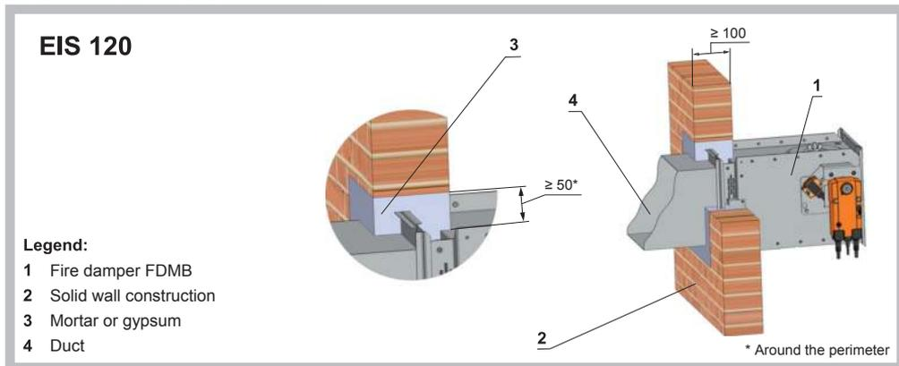
Installation in a solid wall construction
