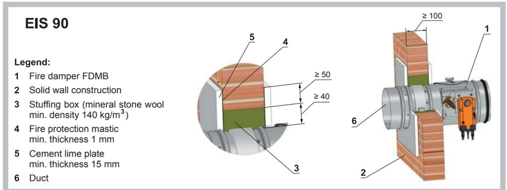
Installation in a solid wall construction (Weichschott system)
