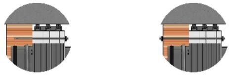
Fig. 45 Solid wall construction - stuffing box, fire protection mastic and cement lime plate
